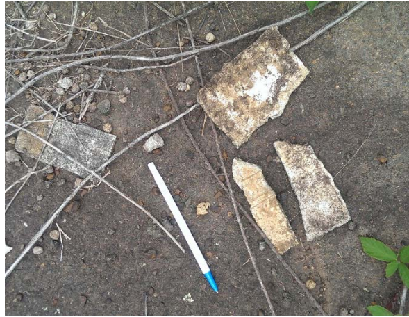
Photograph 14: Suspected weathered ACM fragments observed near radar loop
